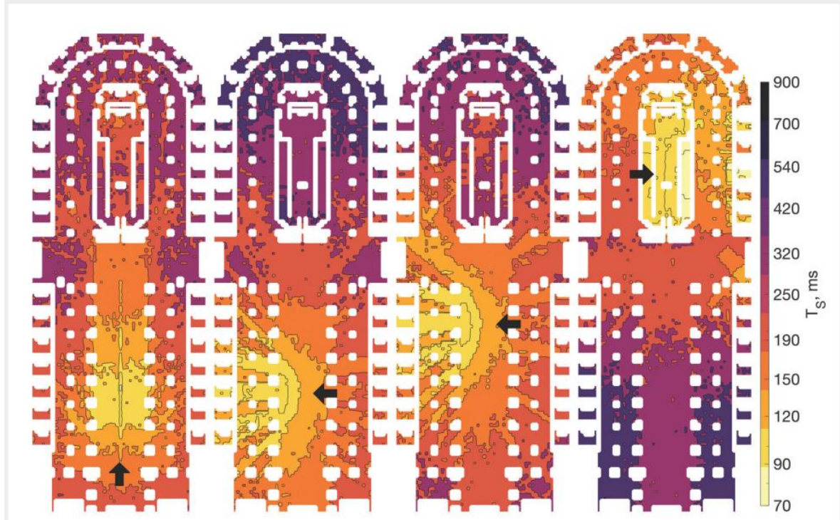
Figure 5. Center time ( T_s ) for unoccupied condition, comparing organ position/orientations (black arrows). Left to right: location of the contemporary grand organ in the tribune; two positions in the nave; and the location of the contemporary choir organ. Lower values indicate earlier arriving energy and hence more musical clarity. Reproduced from Canfield-Dafilou et al. (2023), with permission.
